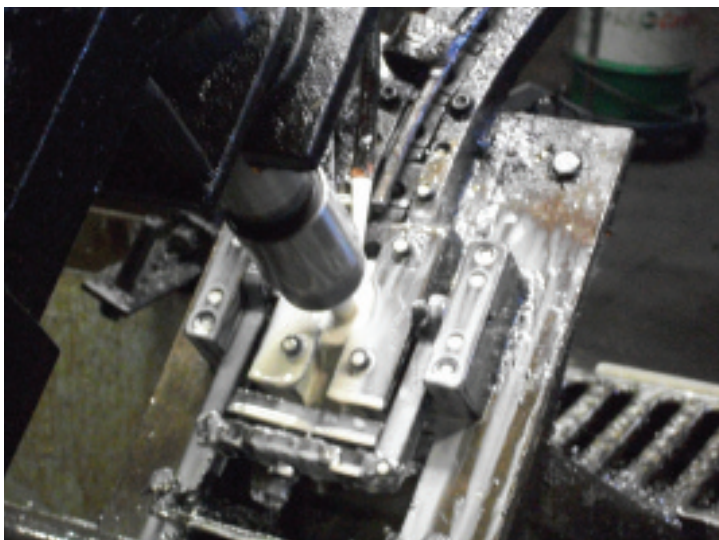
Chemetall’s Tech Cool 35045 metalworking fluid improved tapping life 30% in a test on one nut-tapping head and was expanded to the 11 tapping heads in three nut-tapping lines.
