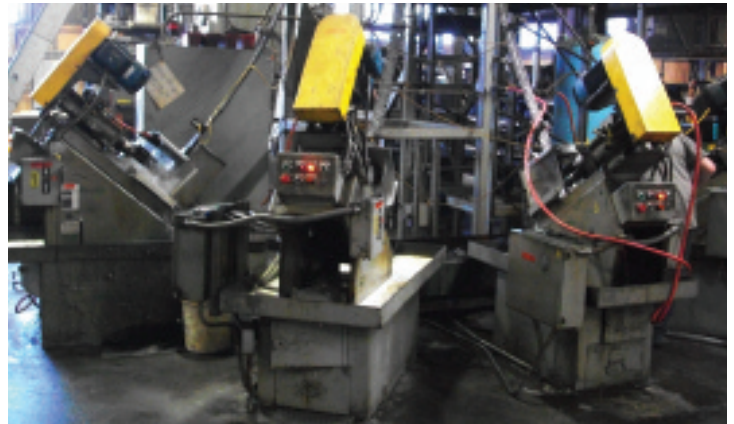
Nut-tapping cells in Unistrut’s Wayne, MI, facility function in an environment that is cleaner, safer, and greener after 85% reduction of oil usage in all operations.
